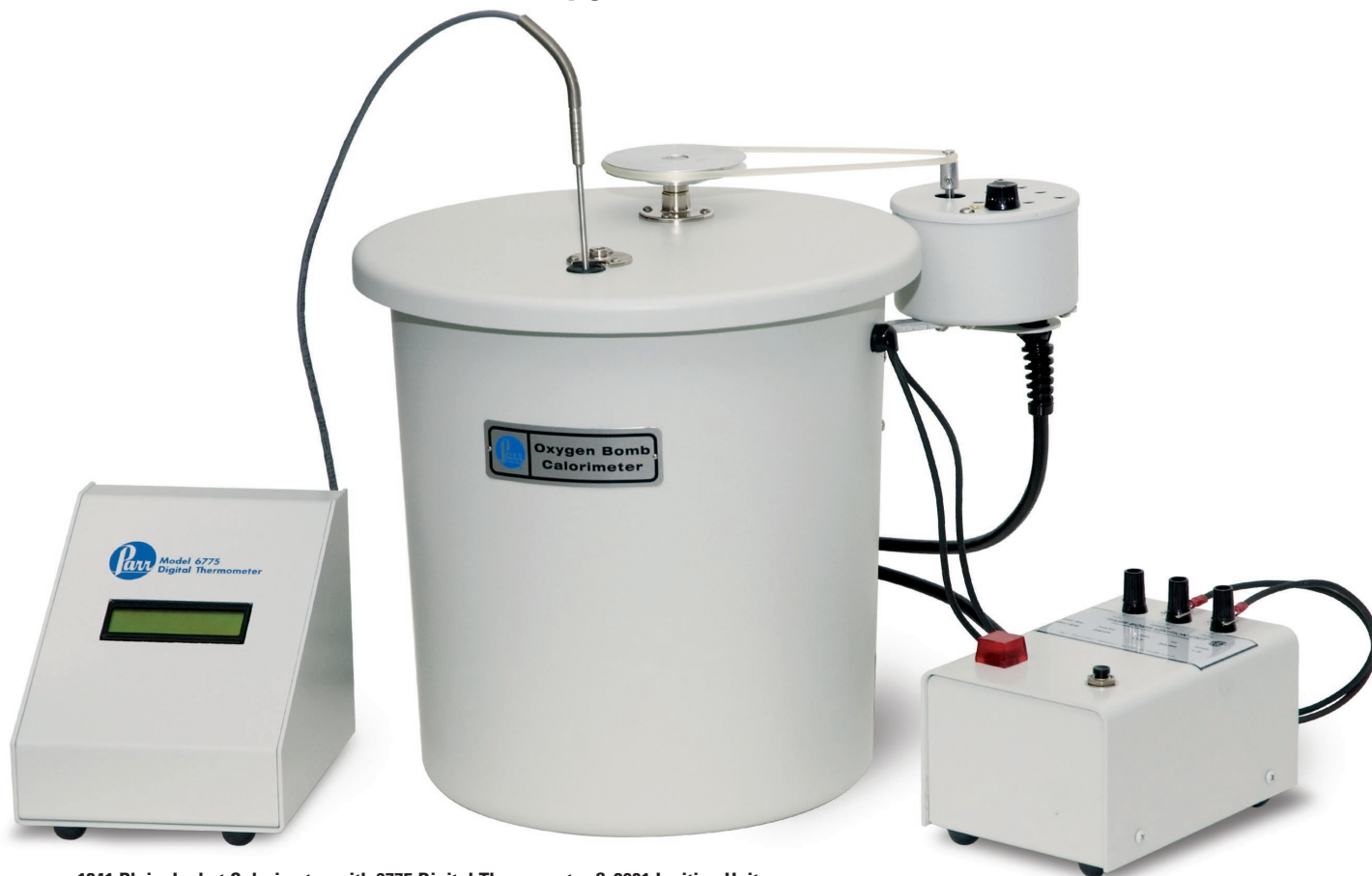
1341 Plain Jacket Calorimeter with 6775 Digital Thermometer & 2901 Ignition Unit
