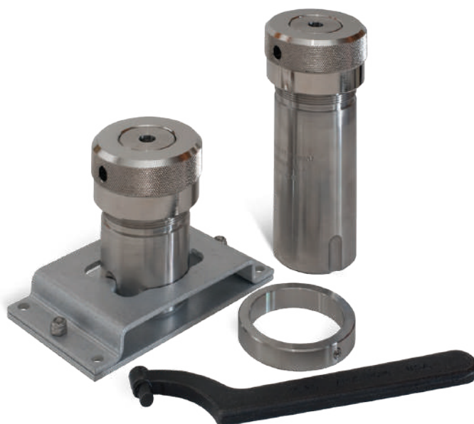
The 4744 and 4749 Vessels can be held firmly in an A285AC Holding Fixture while tightening the cap with a 264AC2 Hook Spanner.
