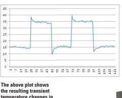
The above plot shows the resulting transient temperature changes in a reactor equipped to perform power compensated calorimetry. The 4547 jacketed reactor used here has an internal volume of 1.2 L and was half full of water. Data were recorded at one minute intervals while the set point bias was toggled 1.5 C. The y-axis is the trim heater power (watts).
