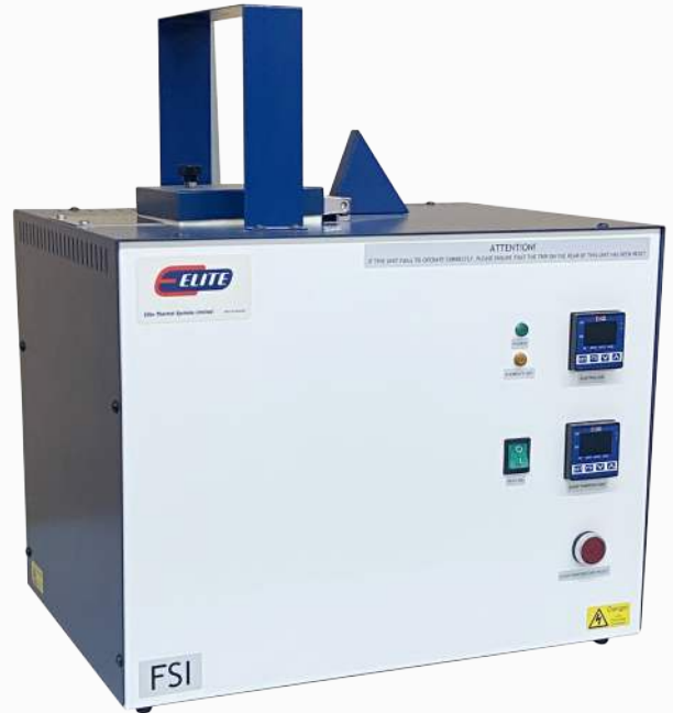
Free Swelling Index Furnace, FSI
